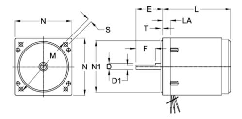
D1 = 7 N1 Diameter = 73 D Diameter = 8 S =  $4x \emptyset 5,5$ E = 32 T = 2 F = 20 Weight (kg) = 1.6 L = 85
